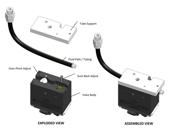
Figure 9. Fluid Path Installation
