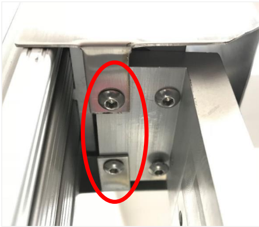
Figure 2. Remove 2 Mounting Screws
