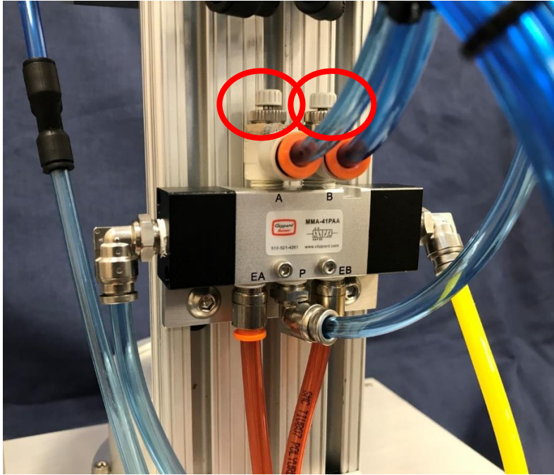
Figure 10. Operating Valve and Flow Controls
