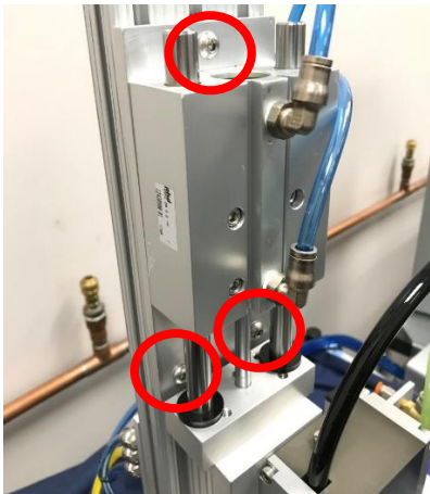
Figure 4. Loosen 3 Bolts on Cylinder Mount Adapter
