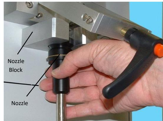
**Figure 12. Nozzle Assembly**
