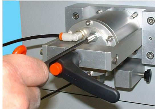
3. Fill a cartridge as you would in normal operation. Observe the fill rate to see if it is acceptable. If the flow rate is too fast, go to step 4; if it is too slow, go to step 5.
