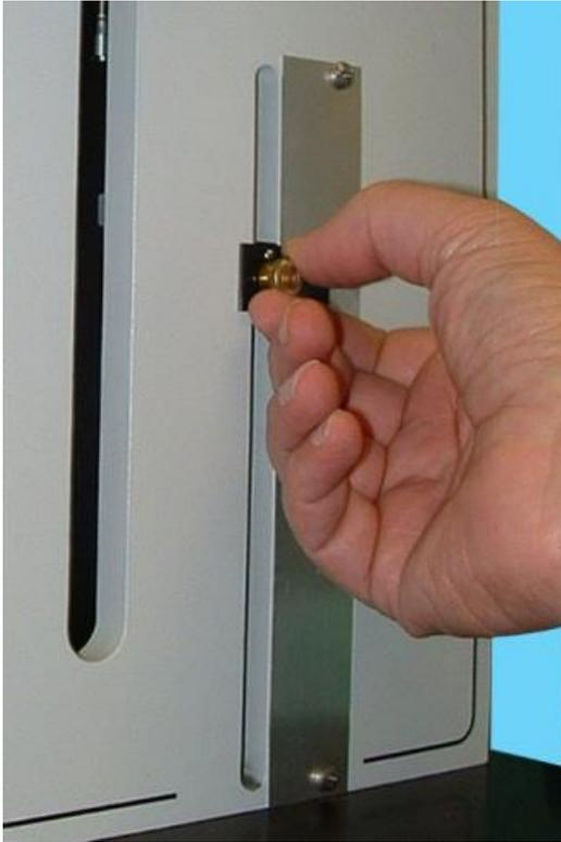
**Figure 14. Cartridge Adjustment**
