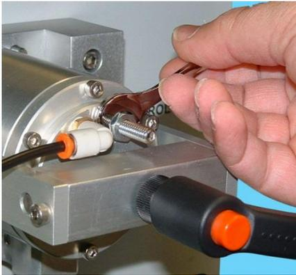
**Figure 16.** Stroke Adjustment Screw
